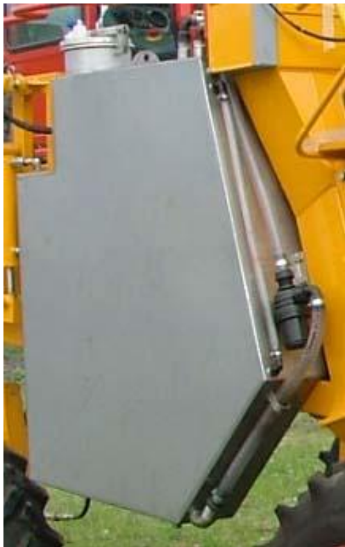
Stainless steel tanks for treatments products from 1000 to 1500 litres capacity (depending on model and configuration)
