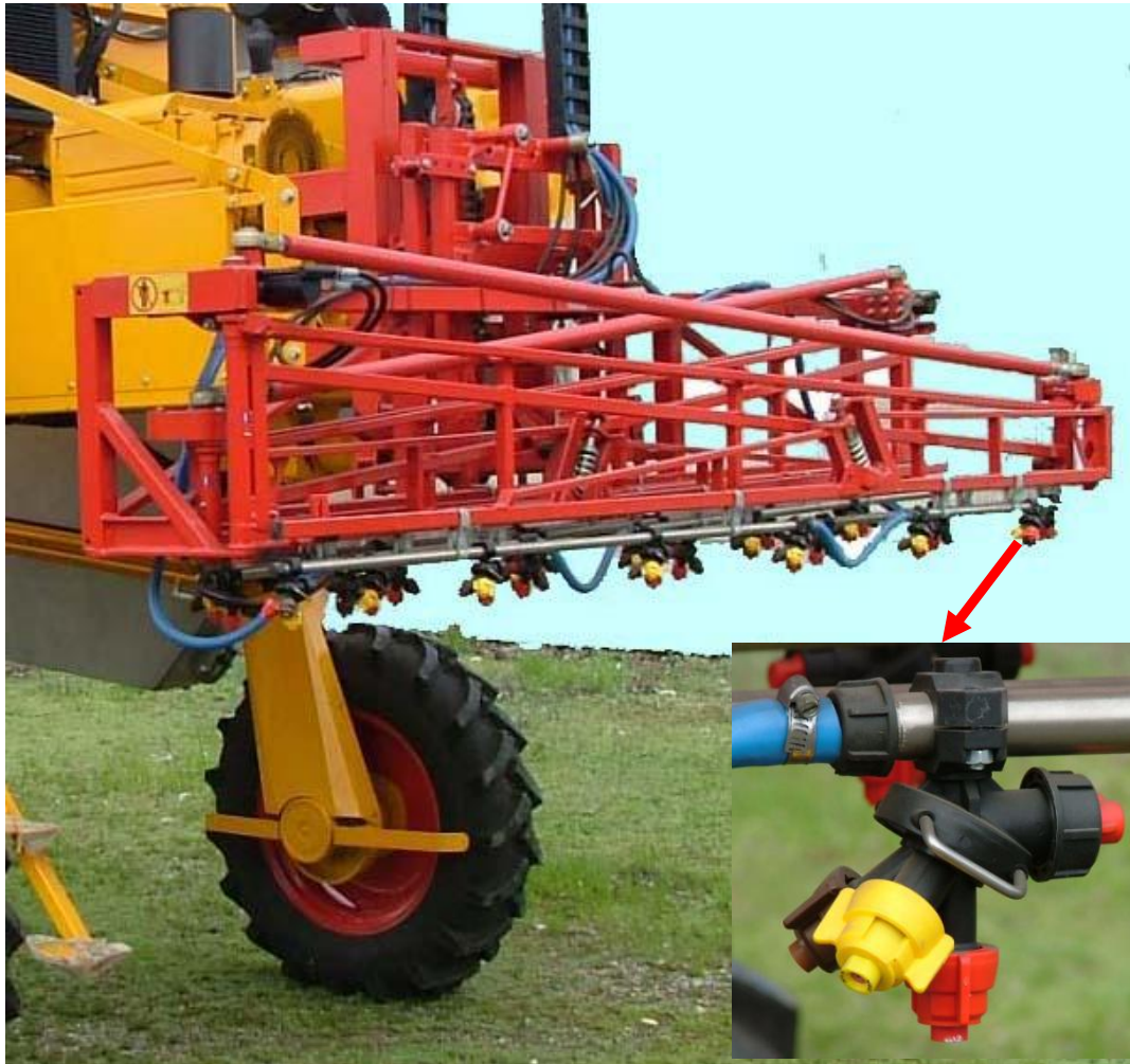
Spraying bar 12 or 15 metres (with full hydraulic system) provided with Tri-Jet noozles
