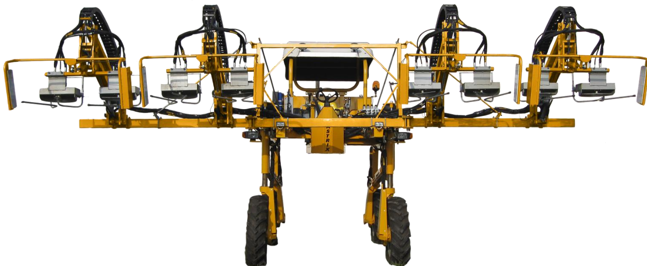
CASTRIX S5 Matic with cutting equipment (knives set to work on 8 rows)
