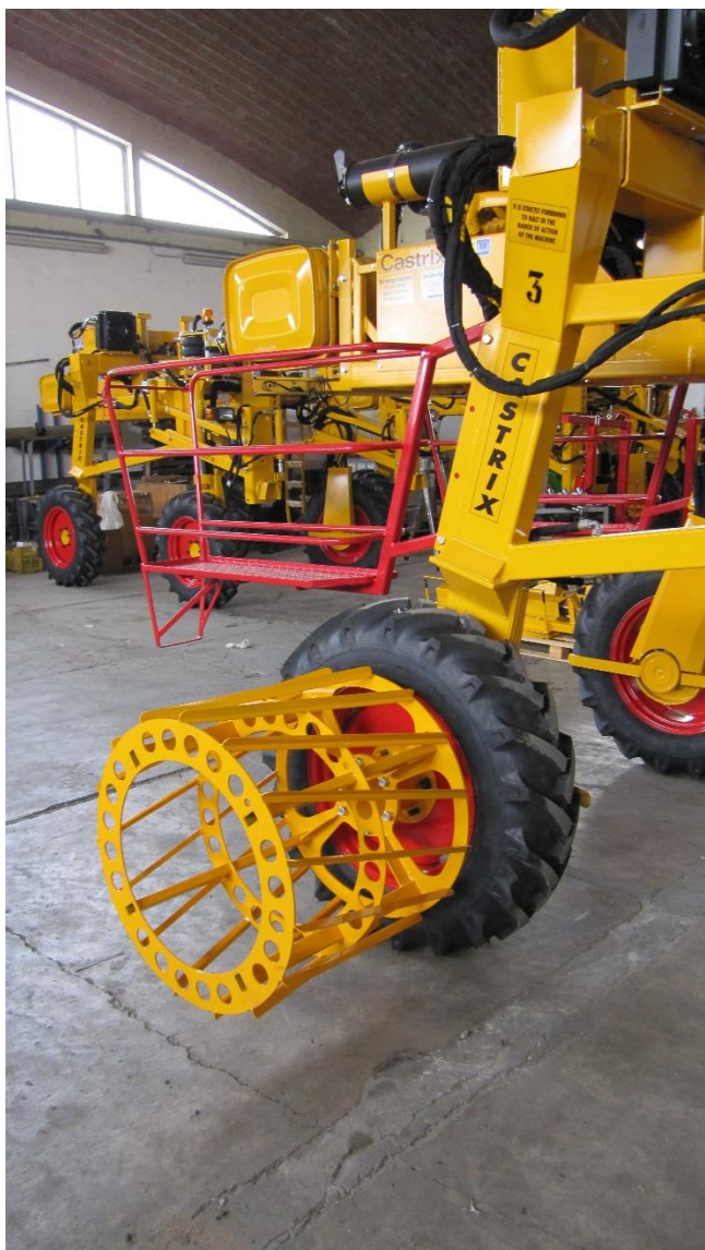
Male row destroyer: mounted on the wheel it allows a quick pass in the field and ensure the complete destruction of the row male
